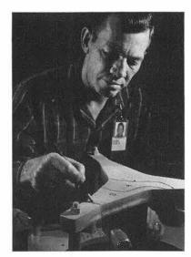
PATTERN OF STRESS is revealed by cracks in the "Stress-coat" sprayed onto handling gear prior to undergoing static test. Eldon Coomes marks the pattern with grease pencil to further aid stress analysis.
